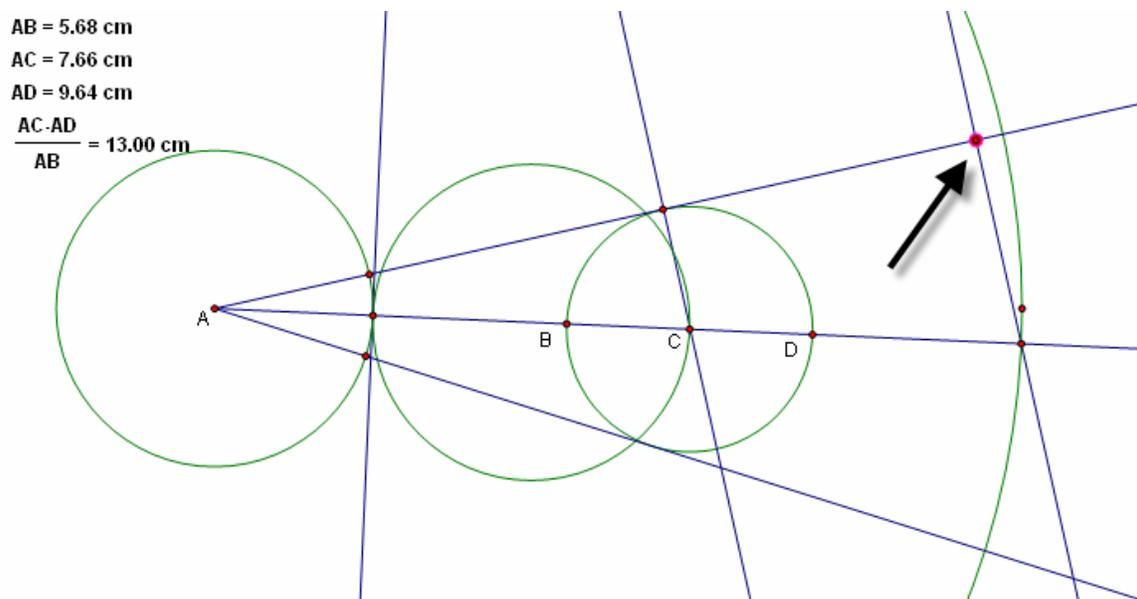
In order, select the new center point and the new point of intersection (see picture) and use **Construct** from the menu bar with the **Circle By Center+Point** option.
