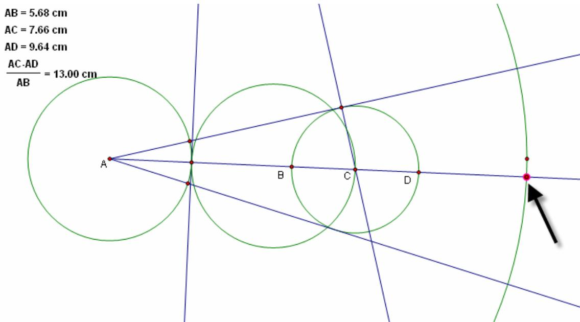
To find the radius of the circle, highlight the new point and the ray that makes the side of the angle. Then use **Construct** from the menu bar with the **Perpendicular Line** option.
