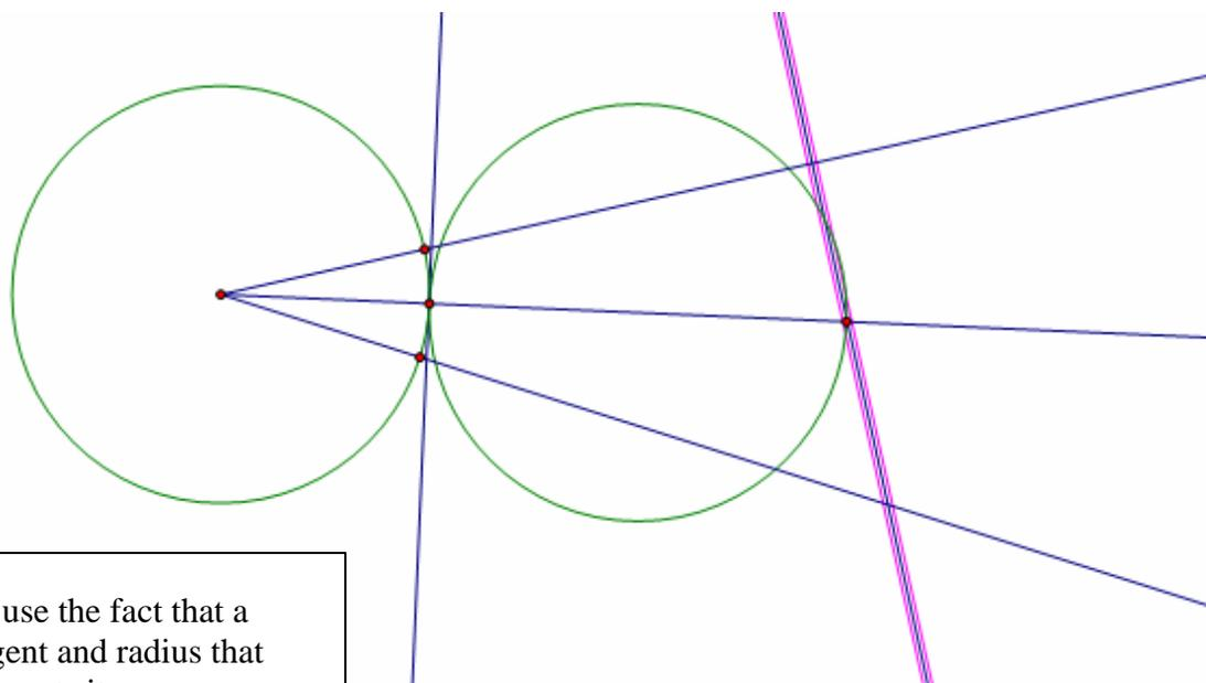
We use the fact that a tangent and radius that intersects it are perpendicular to construct a circle tangent to the rays.
