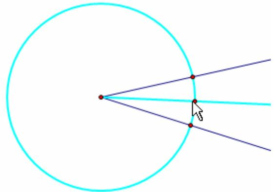
Construct a tangent to the circle through the point of intersection of the circle and the angle bisector by first selecting the point of intersection and the angle bisector, then using **Construct** from the menu bar with the **Perpendicular Line** option.
